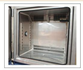
The KMH-L range is a -40°C to +150°C range of environmental chambers available in 5 sizes from 36L up to 1500L. This model features a large 7" full color LCD touch screen controller capable of up to 120 programs or 1200 cycle steps. The programmable controller is easy to use and clear to read making operation simple and quick and designed with ease-of-use a priority.
